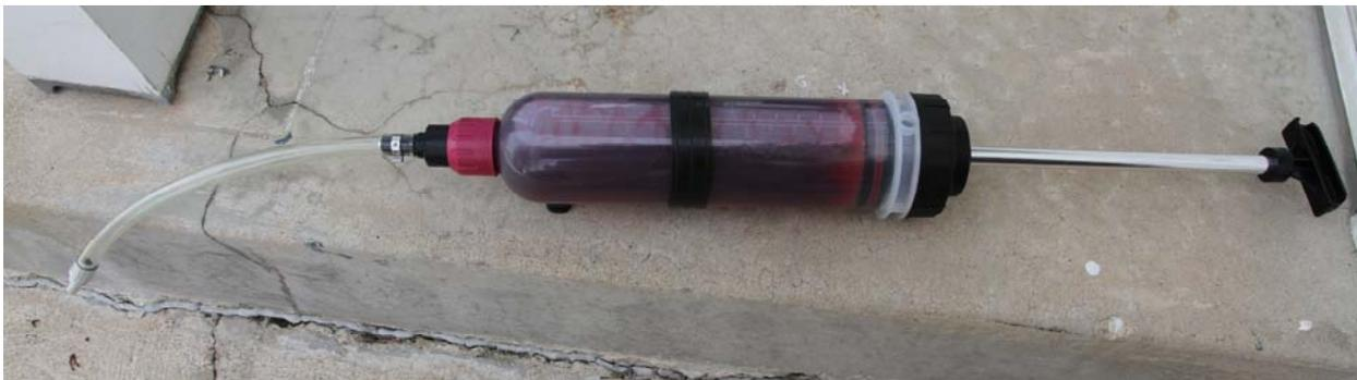
With the pump filled, I was able to slip under the car, poke the end of the hose into the backup light switch opening, open the valve, and fill the transmission back up 1.5 quarts at a time.
